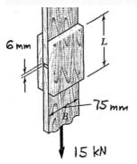
There are four separate areas that are glued. Each of these areas transmits one half the the 15 kN load. Thus
