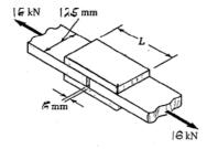
There are 4 separate areas of glue. Each glue area must transmit 8 kN of shear load.
