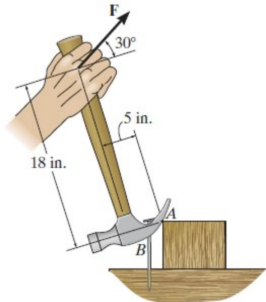
Resolving the 20-lb force into components parallel and perpendicular to the hammer, Fig. *a*, and applying the principle of moments,
