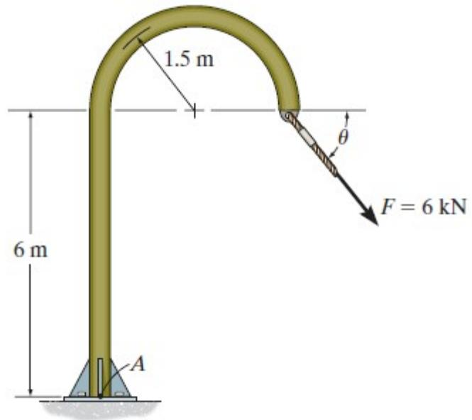
**Moment Function:** Resolving force  $F$  into horizontal and vertical components, Fig. *a*, and applying the principle of moments,
